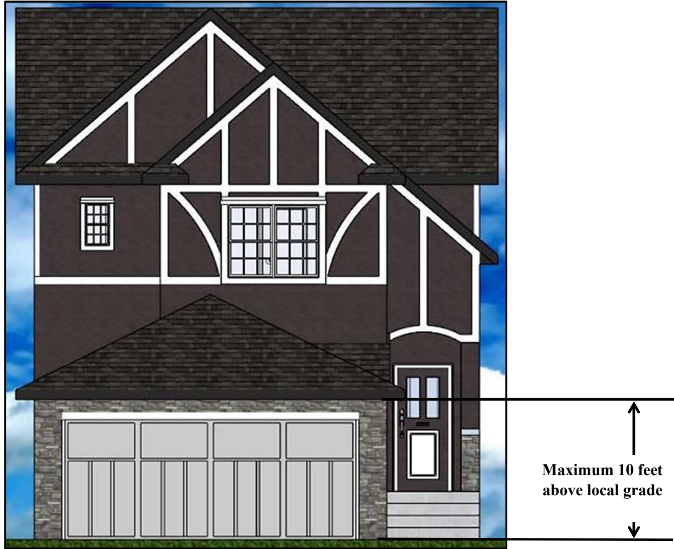
Figure 1: Example of an adhered manufactured stone veneer installation up to 10 feet (3048 mm) on a Part 9 residential unit constructed per 9.10.15 only.
