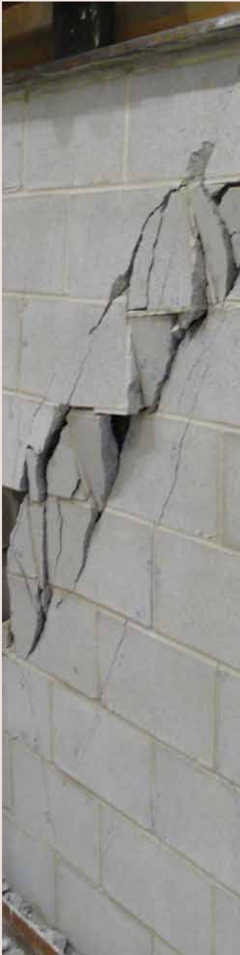
Left: Effects of the different parameters affecting the shear resistance of concrete masonry walls. Wall with no joint reinforcement (vertically reinforced outer and middle cores)
